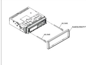
If you want to take CHASSIS out of the SLIDE BRACKET HOUSING, remove the PLASTIC OUTLINE away, then insert the two KEY PLATE into left and right side of chassis as above illustration.
